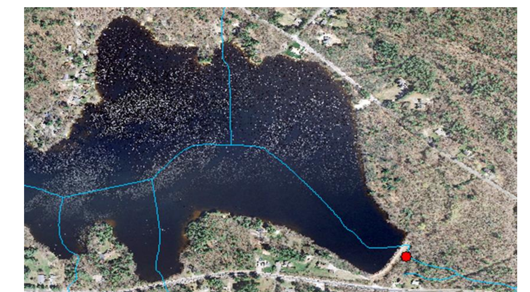
Sample reservoir above a dam (red dot) along flow lines. High resolution digital orthophotos used to confirm the existence of a dam which was then snapped to the river.
